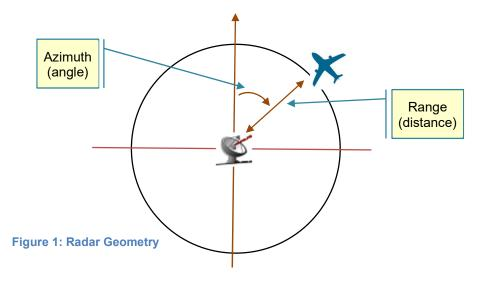
The Bedford radar is unable to measure to altitude, although Whirlwind later incorporated special height-finding radar as well (footnote)
