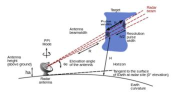
From a mathematical point of view, each echo represents a point on a polar plane, centered at the location of the radar station, with an Azimuth, or angle measured from a reference point (often due North) and a Range, or distance away from the station. Simple trigonometry can convert these polar coordinates into a cartesian x/y plane.
