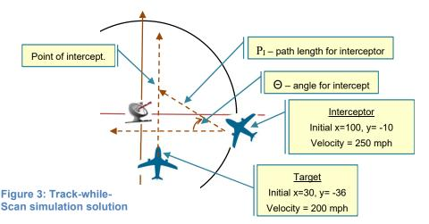
The Whirlwind program solves this trigonometric problem with an iterative algorithm that tries successively smaller time intervals until it finds the angle that will cause coincidence.
